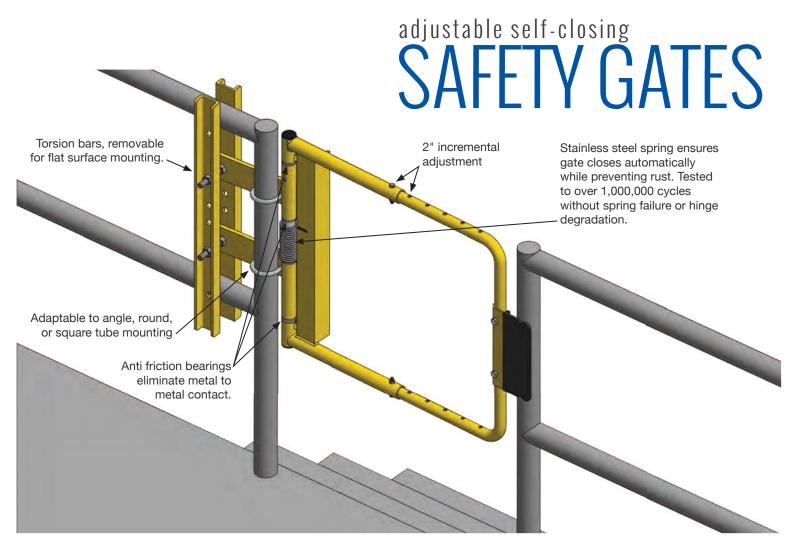
COTTERMAN® ADJUSTABLE SELF-CLOSING GATES can be used as barriers to prevent unintended egress through guardrail openings in accordance with OSHA and ANSI standards.
